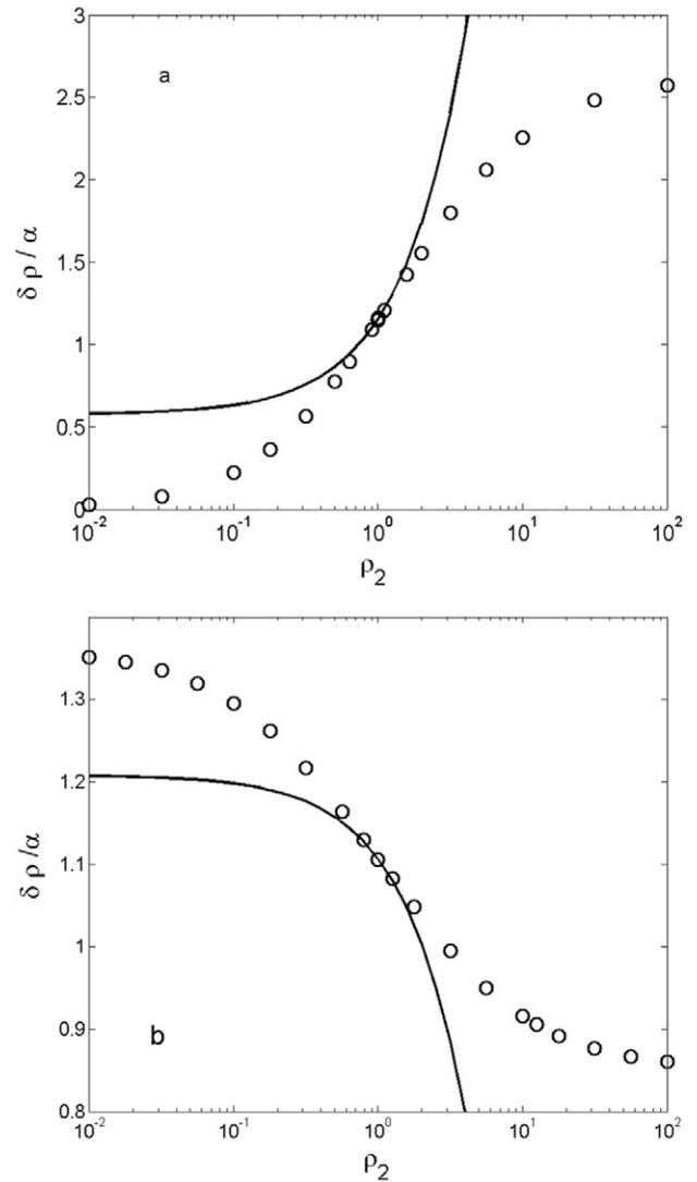
Fig. 5. The relative error in the apparent resistivity as a function of the resistivity in a 2D dyke of width 0.3 (circles). The solid line represents the estimated error predicted using the sensitivities of the various regions when  $\rho_2 = 1$ . The value of  $\alpha$  used was 0.4. a) The 2D dyke is centered on the C electrode b) the 2D dyke is just to the left of electrode A. Positions of the dykes are shown in Fig. 2.
