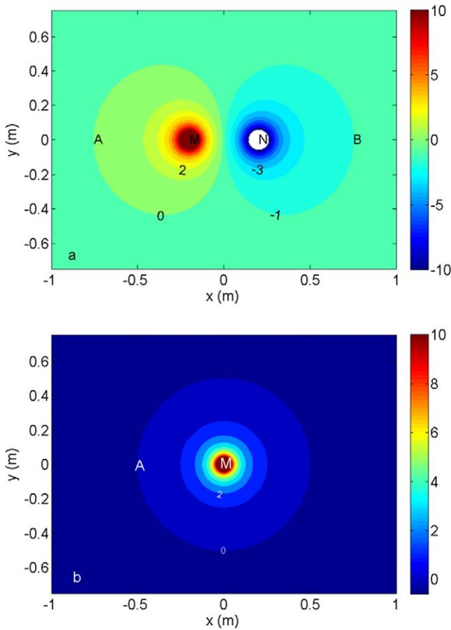
Fig. 4.  $\delta\rho/\alpha$  for a) a Schlumberger array and b) a pole-pole array, where the additional grounding point is connected to electrode A.
