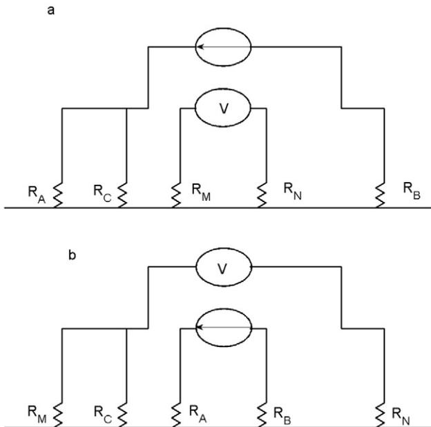
Fig. 1. a) Resistivity array with current leakage on a cable connecting to electrode  $A$  resulting in an additional electrode  $C$ . b) Resistivity array with cable connecting to potential electrode  $M$  grounded creating an additional potential electrode  $C$ . Note that the arrays in a and b are the reciprocals of one another with the substitutions  $A \leftrightarrow M$  and  $B \leftrightarrow N$ .
